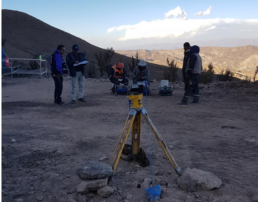
Figure 12.5 Radial Drill Collar Verification at Santa Barbara Hill
